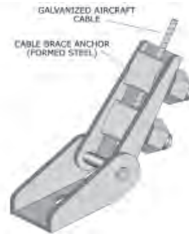
Figure 152: Cable attached with bolts to a bracket.
