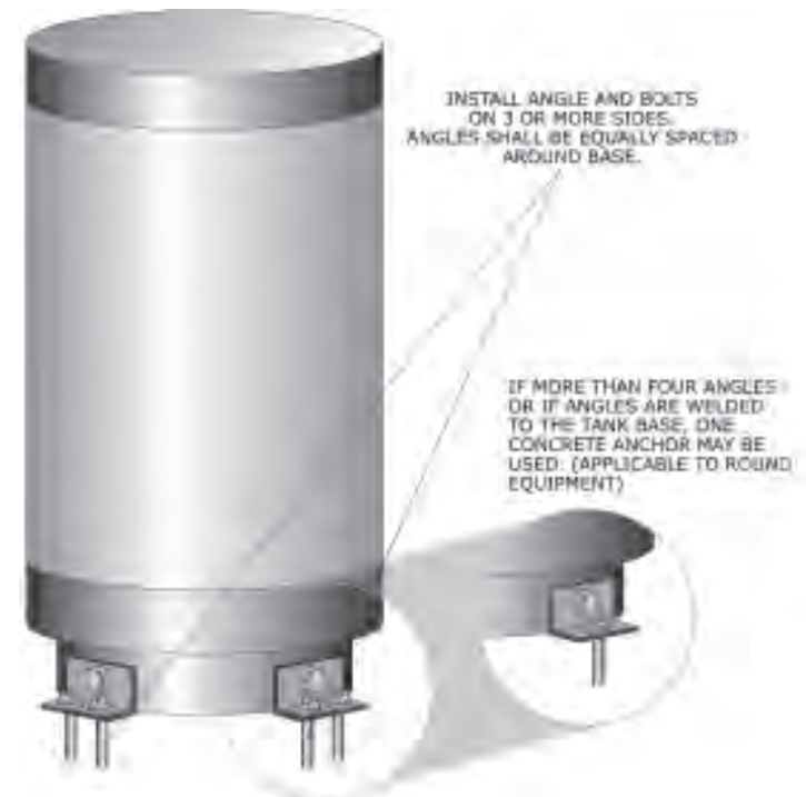
Figure 76: Three or more angles used to bolt down equipment with a round base.
