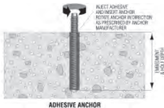
Figure 134: Adhesive anchor installation.
