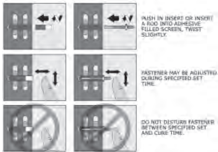
Figure 144: Brick wall adhesive anchor.
