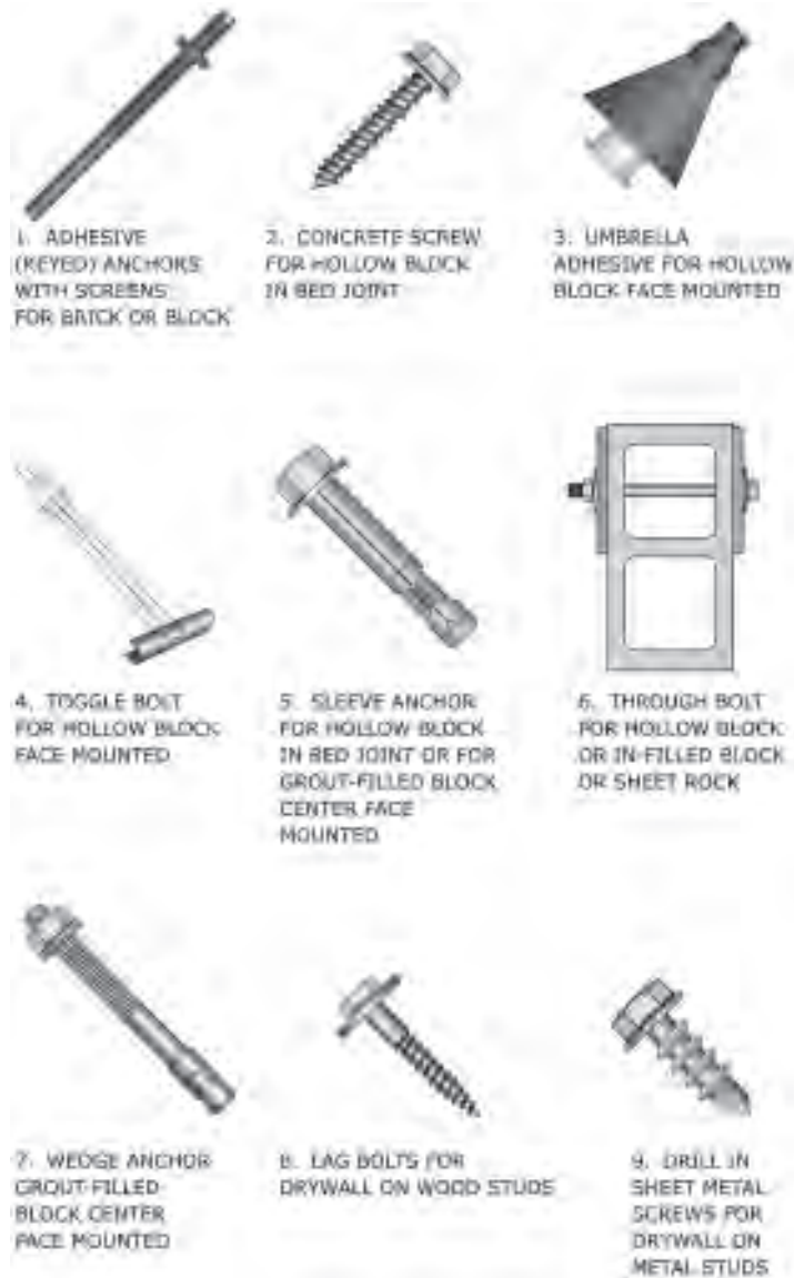
Figure 141: Types of masonry and drywall anchors.
