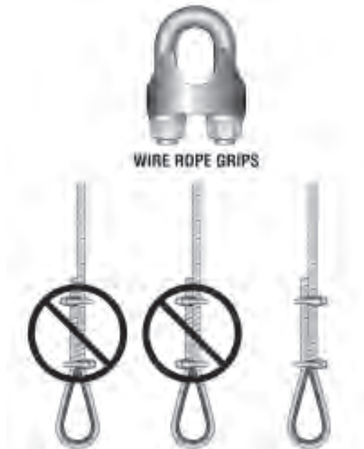
Figure 155: Wire rope grip assemblies.
