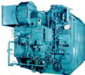
Figure 21: Water-tube (shown) or fire-tube boiler.
