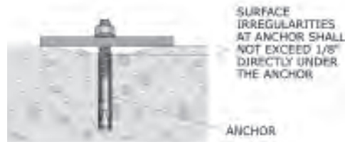
Figure 137: Acceptable gap for grouted plate.
