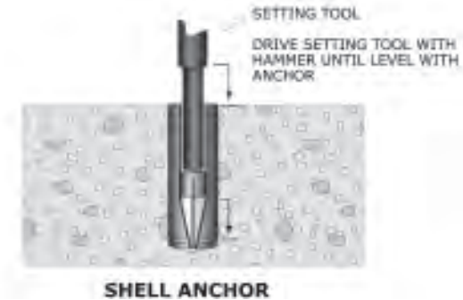
Figure 135: Set shell anchors.
