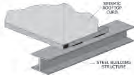
WELDED DIRECTLY TO BUILDING STRUCTURE
