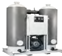
Figure 5: Skid-mounted equipment including large filter dryers.
